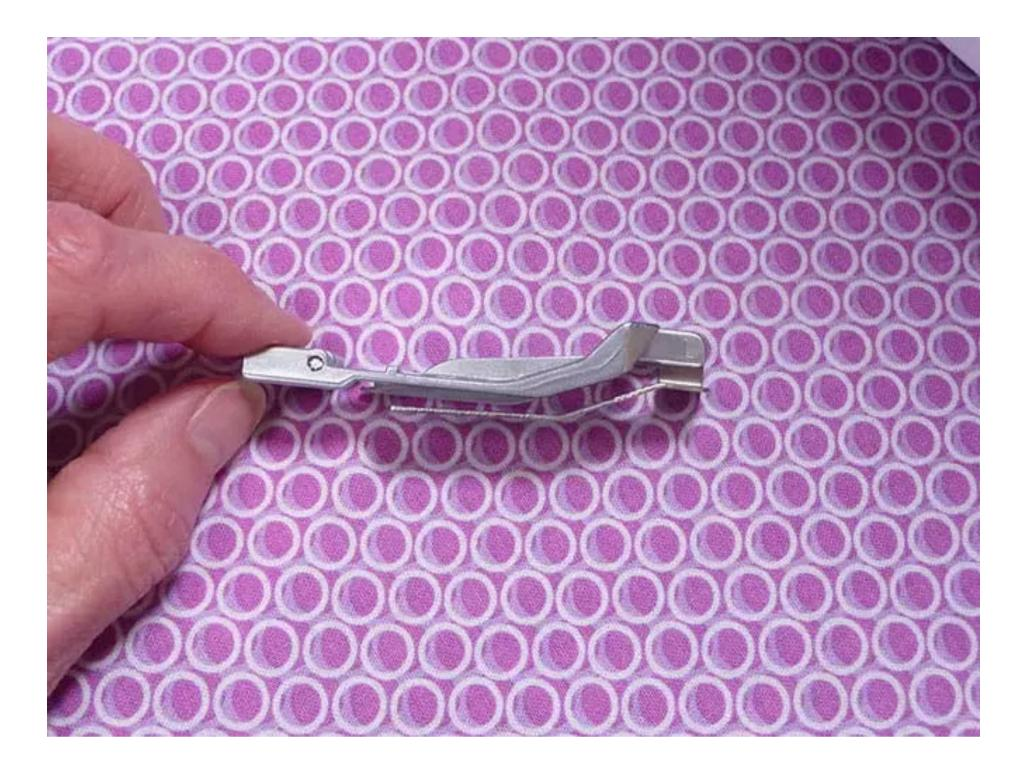
Here's how the foot is designed to work: Place the fabric you want gathered against the feed dogs, having the fabric right side facing up, and positioned under the plate. This fabric can be a single or double layer. In this project we're using a double layer folded strip of fabric for the ruffle. This bottom fabric piece comes in contact with the feed dogs and is gathered due to the settings put in place in step 3.
