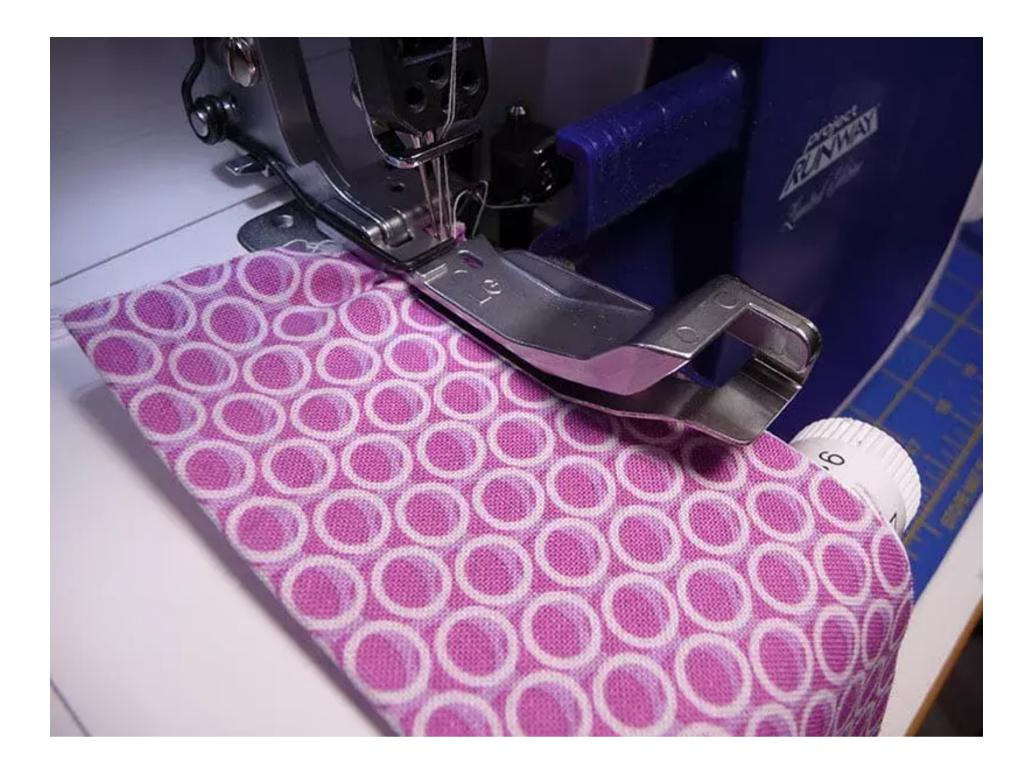
Next, slip the base fabric, fabric #1 into the open slot of the foot, between the separator plate and the bottom of the foot. The plate keeps the fabric from coming into contact with the feed dogs, so this piece is kept smooth and not gathered.
