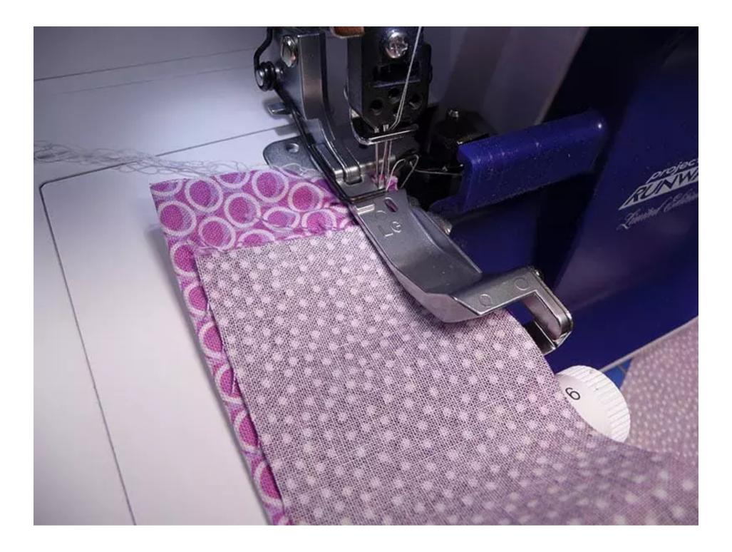
With these two fabrics placed properly in the foot, bottom layer will gather at the same time it's stitched to top layer. In addition, all layers are edge finished and stitched together in one quick step.
