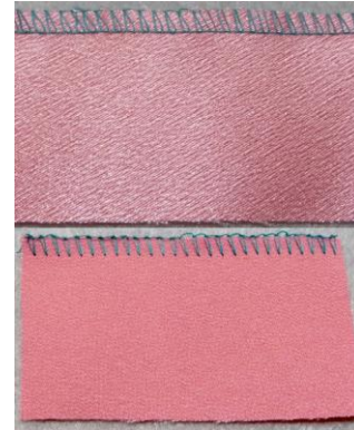
Two thread overcast stitch with standard thread.
