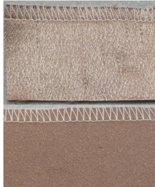
Three thread overlock with standard weight thread.
