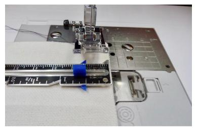
Start with a straight stitch in the left needle position. Next, I find a guideline on the plate that I want to follow. In this case I selected the first line closest to the foot. I choose this line regardless of the metric or inch marking, selecting it merely for convenience. It's an easy sight line to follow because it is the very first line past the presser foot. Now, I set my seam gauge for the desired distance and place it along the raw edge. In this example I want to stitch a 1/2-inch seam.
