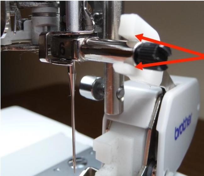
This arm must wrap around the needle bar when you mount the foot on the machine.
