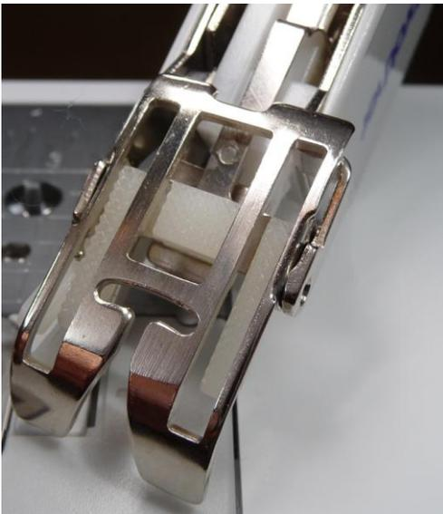
Turn the foot upside down and you can see a view of the teeth built-in to the WALKING FOOT.
