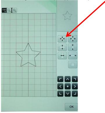
3. To save the star for later touch the memory pocket with the red arrow going into it. Save the stitch to the USB. My star was saved into USB memory, which automatically puts it into the bPocket folder. Touch Preview. Select the double straight stitch option. I suggest changing the stitch length (Run Pitch) to 1.8 to create a slightly shorter, stronger stitch. Touch OK to generate the stitches.
